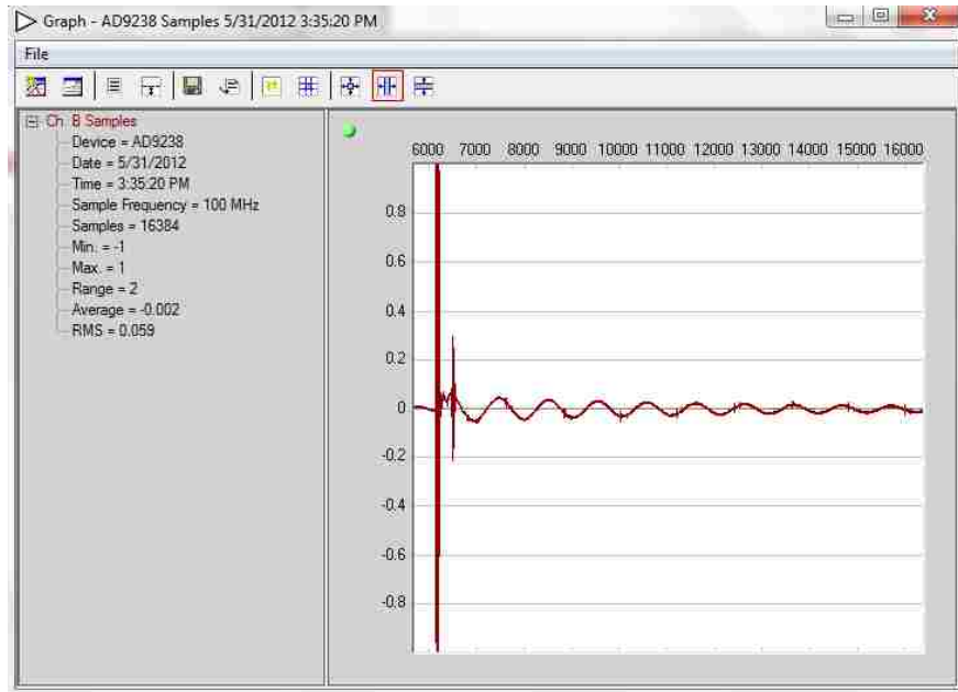
Figure 18: Real-time ADC display of signal using VisualAnalog
